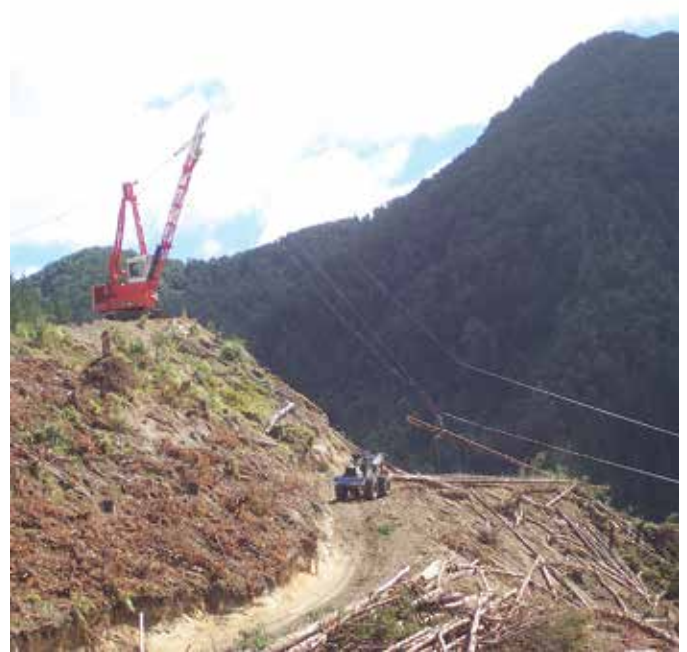
Split-level landing with stems two-staged back to a processing site
