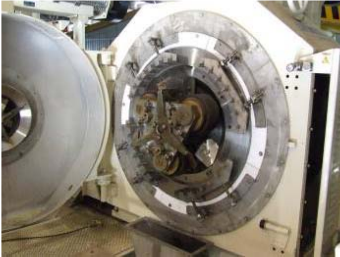
Andritz Pellet Presses - 4t/hr each
