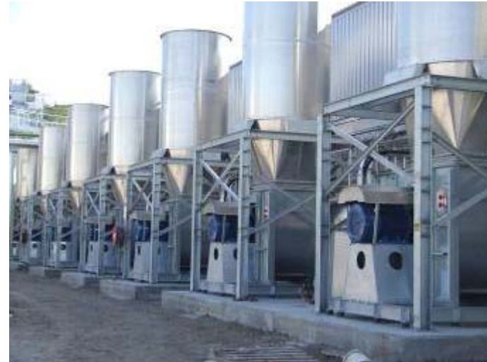
Stela Low emissions belt dryer - 12t/hr
