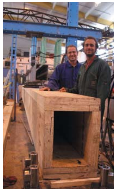
Researchers with a Pres-lam beam Cables running through the void are tensioned when the building frame is assembled
