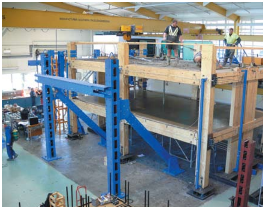
The two-thirds scale Pres-lam building frame being readied for seismic testing at Canterbury University
