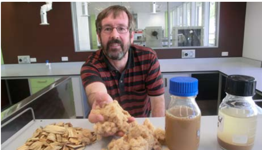
Scion scientist Ian Suckling with the results of the lignocellulosic biofuel initiative L to R: wood chips, wood fibre, pre-treated substrate and soluble sugars in solution, together with lignin and undegraded carbohydrate
