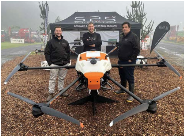
↑ SPS Automation’s new generation of heavy-lift spot spraying UAVs allows for more precise chemical application across forestry operations
