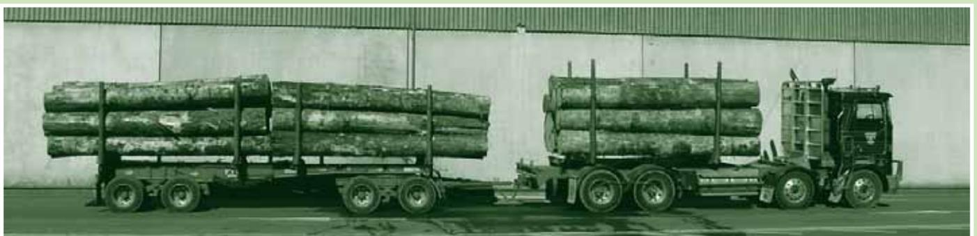
**53-tonne, double-bunk trailer** – Proposed typical 22-metre rig load
