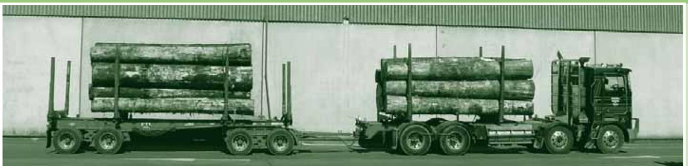
**44-tonne, single-bunk trailer** – Existing maximum 22-metre rig load
