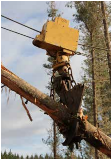
The new Alpine Grapple Carriage: Provides improved control under NZ conditions
