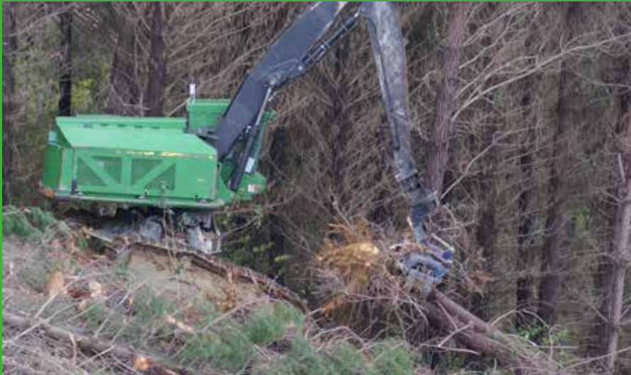
The John Deere operating on the slope with the operator 100 metres away
