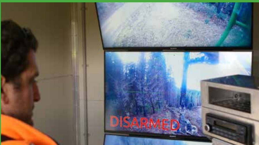
The operator controlling the John Deere guided by the remote camera video
