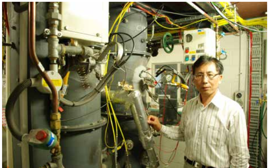
Prof Shusheng Pang with the steam gasifier developed and in operation at Canterbury University since 2007 . He and his team are getting closer to their goal of developing a plant that will enable a medium to large sawmill to use wood waste to meet all its energy requirements and produce bio-fuel for sale
